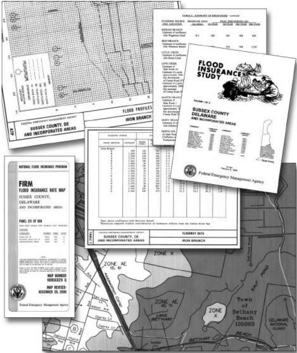
Figure 4-1. Portions of an FIS and a FIRM.
